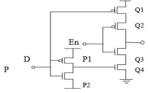
Figure 2: Tri-state Buffer [2]
