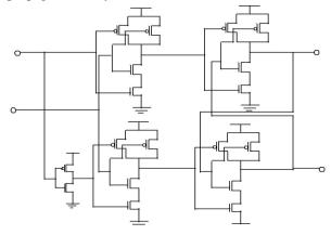
Figure 1: D Flip-Flop [2]
